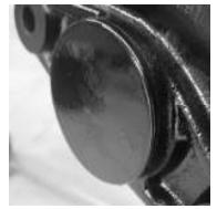
Make sure that both surfaces are thouroughly cleaned with mineral turpentine before the "Selastic" is applied. Using "Selestic" ensures that should the output shaft seal leak pressure acting over the area of the cover is sufficient to force the cover away from the housing thereby avoiding applying pressure to the end of the shaft. When installing the steering gear make sure that the metal cover does not foul the mounting bracket of the vehicle frame.
