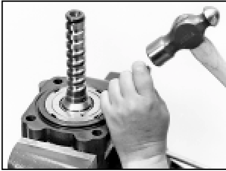
Stake valve housing and locknut
