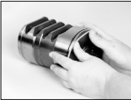
Install rack piston o-ring and seal ring
