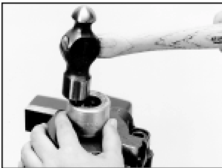
Install input shaft seal
